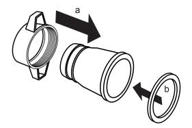
6. Thread the Hose Coupling Ring clockwise onto the Discharge Port until tightened securely.
